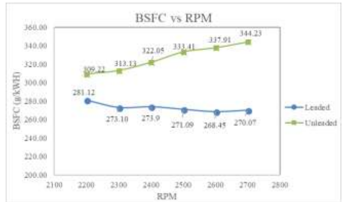
Figure 4: Brake Specific Fuel Consumption of test engine using Leaded and Unleaded Avgas.
